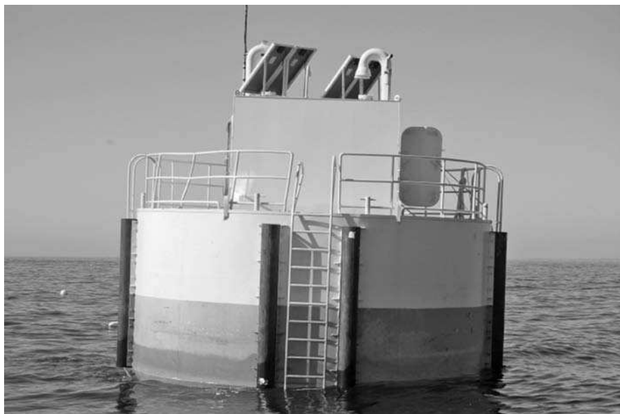
Figure 7.11 A photo of the multi-cage automated feeding system developed by the University of New Hampshire and Ocean Spar at the university's experimental open-ocean farm.
