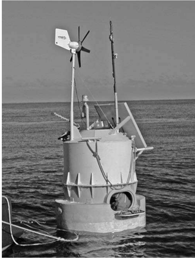
Figure 16.10 A enclosed net pen with monitoring and energy generation. Photo courtesy of the Atlantic Marine Aquaculture Center, University of New Hampshire.
