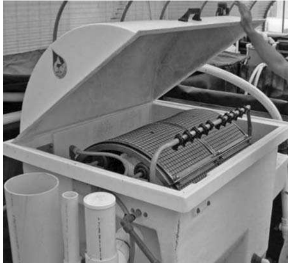
Figure 11.3 Rotating microscreen filter and spray bars for cleansing.
