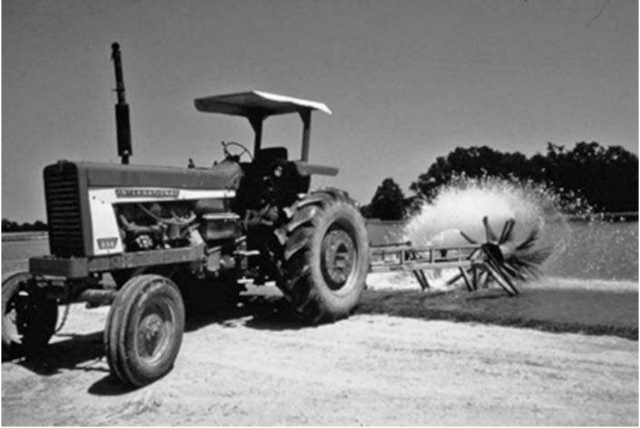
Figure 10.5 A tractor-powered paddlewheel aerator. This paddlewheel directs water parallel to the pond embankment. Other designs push aerated water away and perpendicular to the embankment. Photograph courtesy of E. L. Torrans, United States Department of Agriculture.
