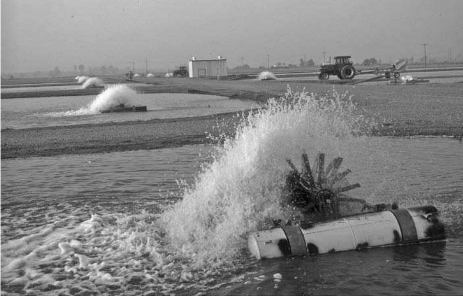
Figure 10.6 A floating, electric paddlewheel aerator. Note the splash pattern and the zone of oxygenated water adjacent to the aerator. Photograph courtesy of E. L. Torrains, United States Department of Agriculture.
