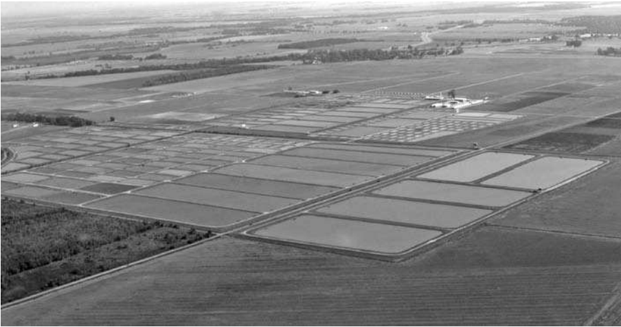
Figure 10.1 Embankment ponds at a large aquaculture research facility in Mississippi. Pond sizes range widely within this facility because the best size depends on research needs. Ponds in the foreground are approximately 4 ha, which is the average size of embankment ponds used in commercial catfish farming. Photograph courtesy of Danny Oberle, Mississippi State University.
