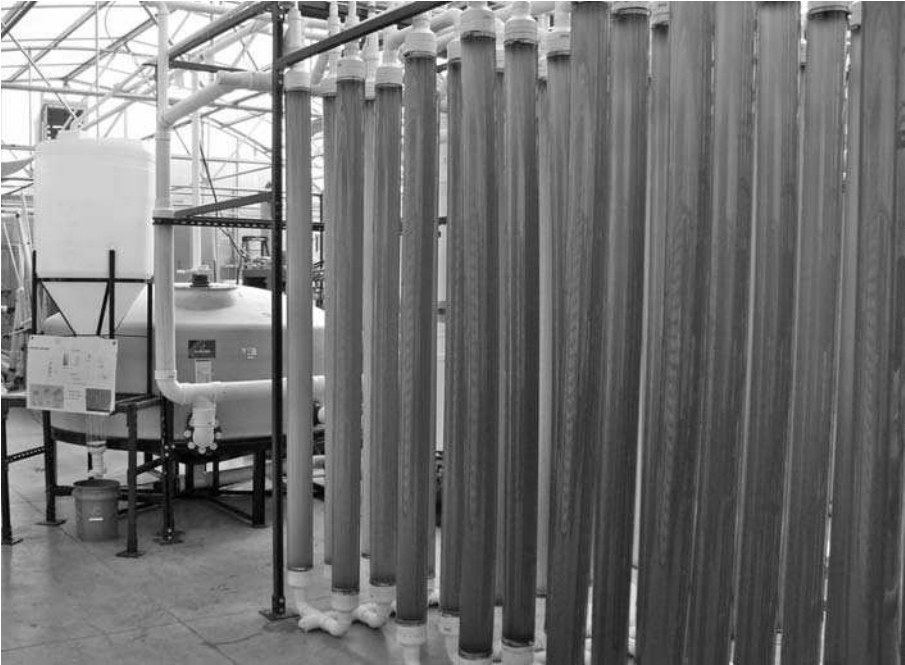
Figure 16.12 Photobioreactors for raising algae. Photo courtesy of Sam Morton, Center for Applied Energy Research, University of Kentucky.
