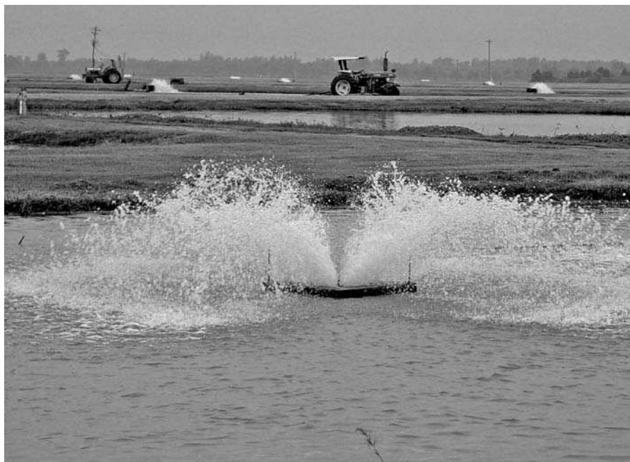
Figure 10.7 An impeller-type vertical pump aerator. A submerged electric motor drives an impeller that throws water into the air. This type of aerator is especially suited for small ponds. Photograph courtesy of E. L. Torrans, United States Department of Agriculture.
